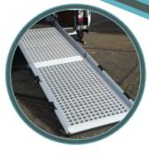
The SE folding Ramp is specially developed for low-floor buses and can be operated by hand or electronically for easy vehicle access. Weighing just 16kg for the manual version and 36kg for the electric version, SE Ramp works perfectly on all vehicles including EV.
