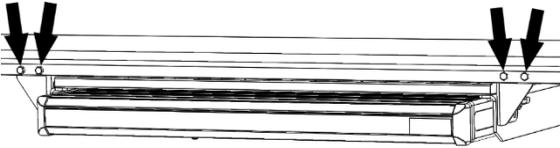
Take the flexible mounting brackets supplied with the step. These brackets can be mounted in several ways. The brackets should be used to fix the rear side of the step to the bottom of the vehicle. It is recommended to find a strong point at the vehicle floor. Mount the brackets in such a way that they bridge the gap between step and vehicle floor / chassis.
