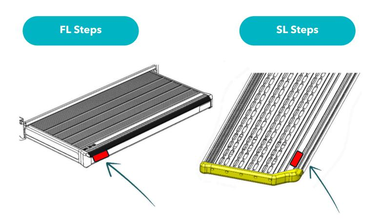
If the serial number sticker cannot be found in this location a serial number 'plate' can be found elsewhere on the step.
