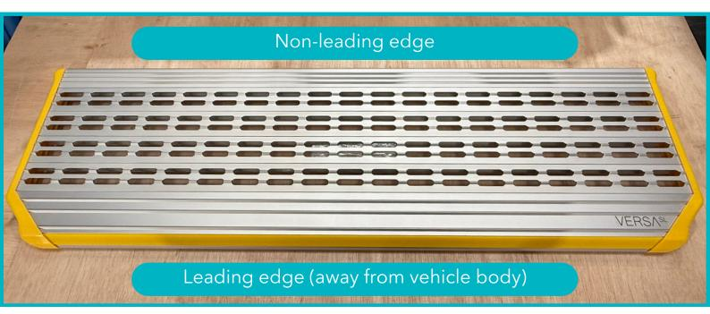
Viewed from underneath step serial number plate is affixed at the leading edge of the step.
